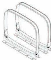
Rear mounting kit with two brackets and stainless steel straps (40mm)
